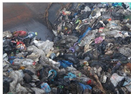
Plastics sorted out from mixed municipal waste contains high levels of organic contamination
