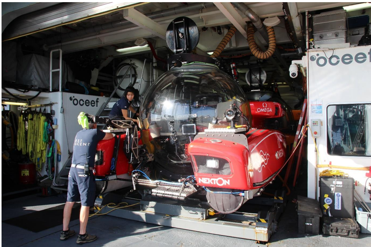
Figure 2. Triton 3K3 submersible undergoing preparations for diving during the expedition. The hydrolek arm is in an upright position (yellow cloth for visibility) and both survey and pan and tilt cameras visible.
