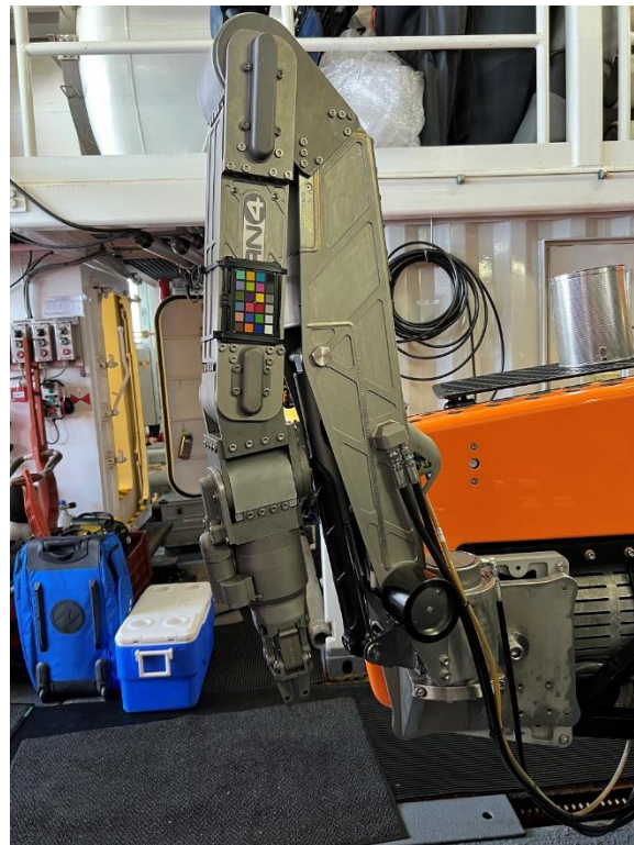
Figure 43. Titan T4 Arm showing mounted colour correction chart.
