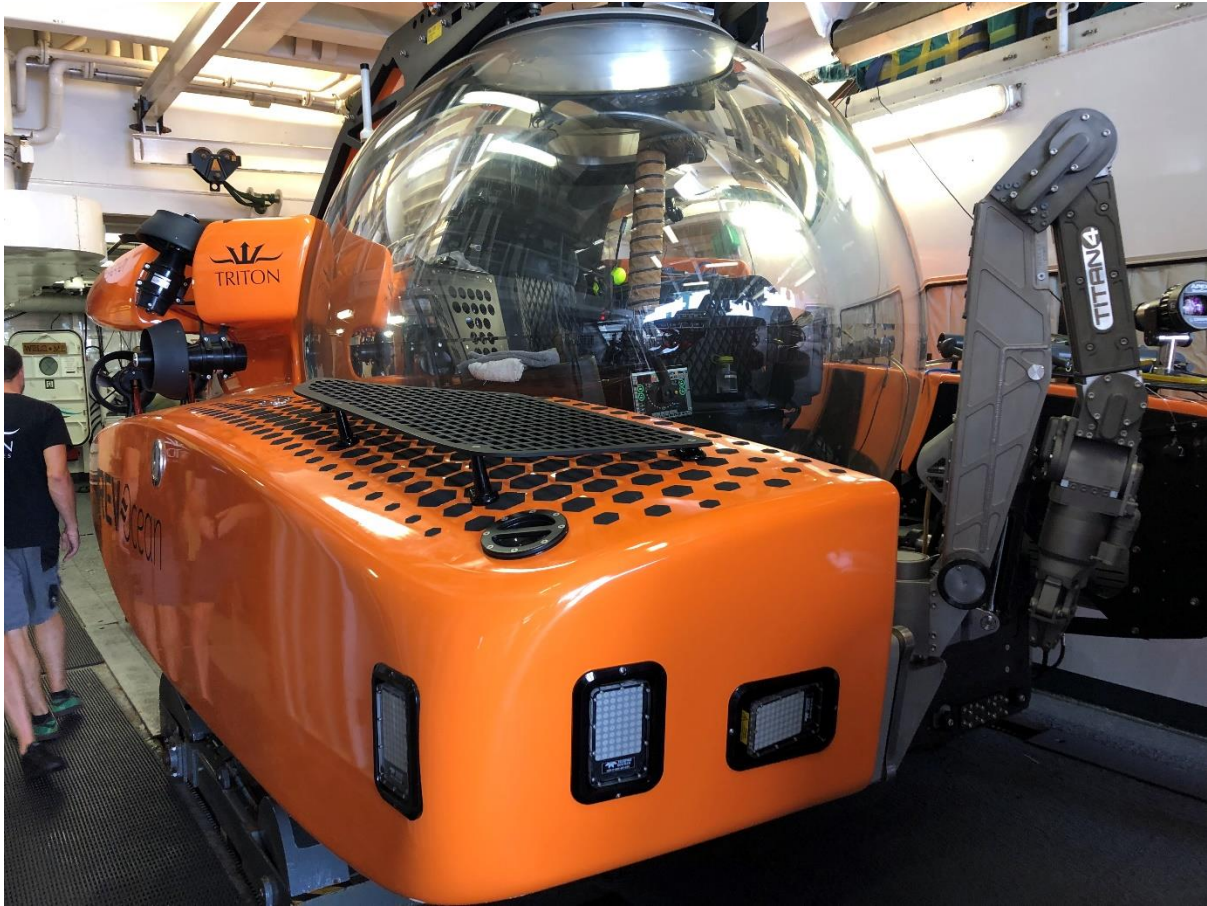
Figure 3. Triton 7K3 submersible, Aurelia showing the Titan 4 hydraulic arm, the prime tool used for sampling deep-sea organisms during the expedition.
