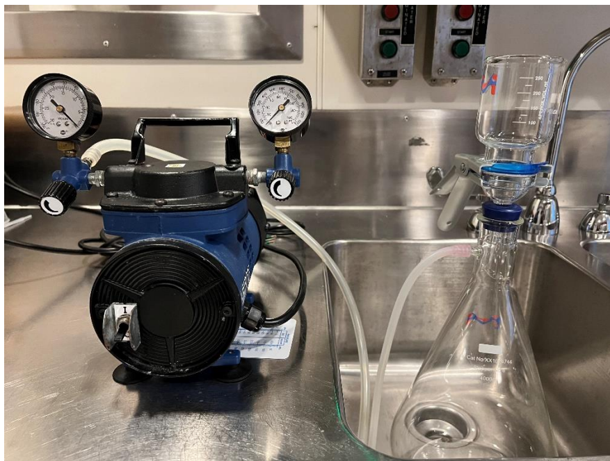
Figure 10. Millepore pump setup for filtering seawater samples for eDNA analysis.
