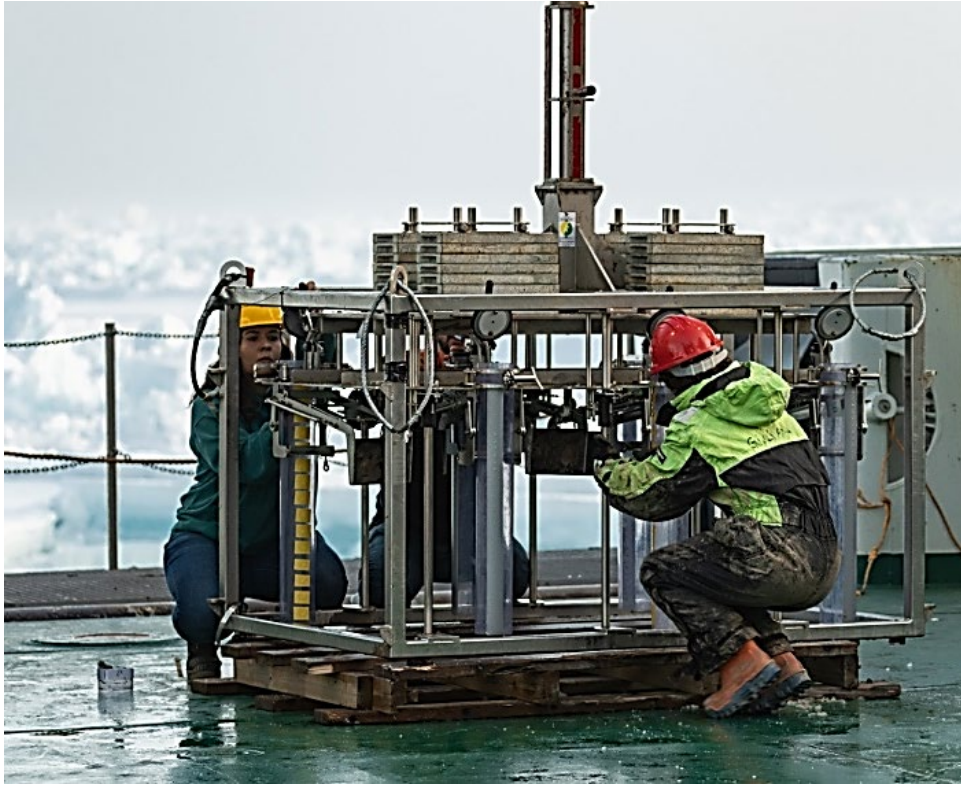
Figure 10.2. Rigging the liners on the multicorer on deck.
