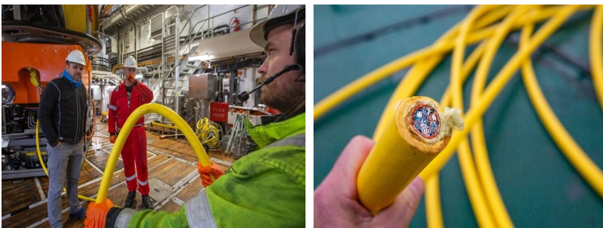
Figure 17. Repair of the ROV's umbilical tether.
