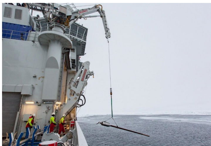
Figure 32. Gravity corer pulled on deck after sampling
