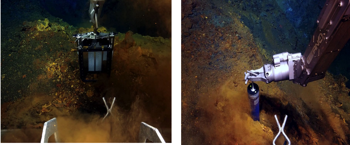
Figure 22. Sampling sediment with the blade corer and a pushcore.
