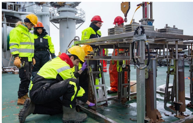
Figure 31. Multicorer on deck with six sediment cores.
